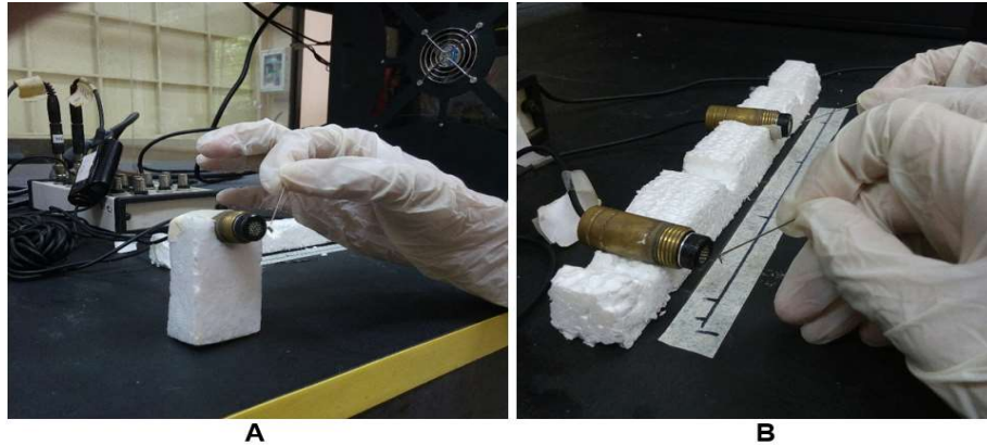
Figure 5A-B. Pressure-gradient microphones placed at a 1-cm distance from the tethered mosquito (A) and at varied distances (1 cm, 7cm, 13cm, and 19cm) for the duet group (B)
