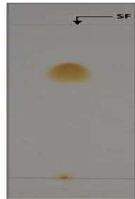
Figure 2. Thin layer chromatogram of purified MFPP or methanol fraction of P. pellucida L. HBK. Solvent System -Methanol:Acetone:5:95. Spots visualised under iodine vapour.
