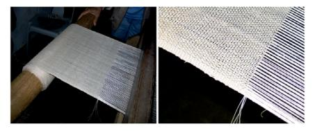
Figure 8. Neatly woven *sinamay* from the multi-stranded abaca yarn.
