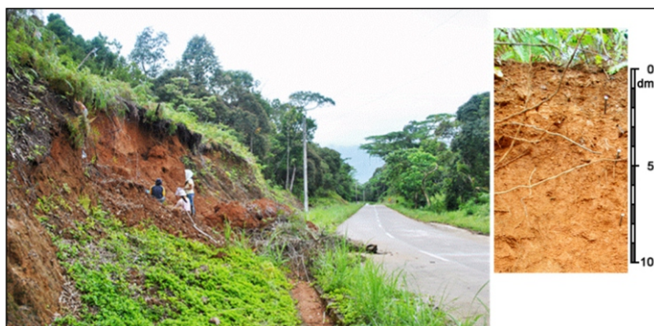
Figure 8. Photographs showing site (left) and profile characteristics (right) of soil profile 5 located at the summit position at 369 m asl in Imelda, Silago, Southern Leyte
