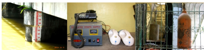
Figure 5. Water gauge level (1), two-way battery-operated radio (2) and bells (3) used for early warning in Brgy. Cogon
