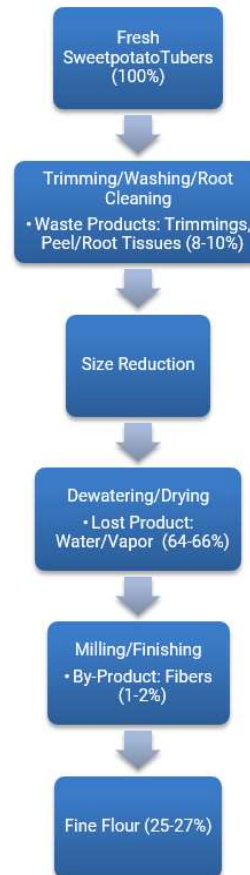
Figure 2. Process flow and material balance in sweetpotato flour processing
