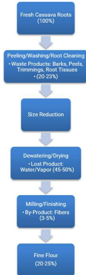
Figure 1. Process flow and material balance in cassava flour processing
