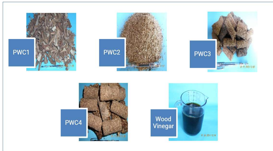
Figure 4. Processing wastes raw, as prepared into different fuel feed forms and the output product wood vinegar
