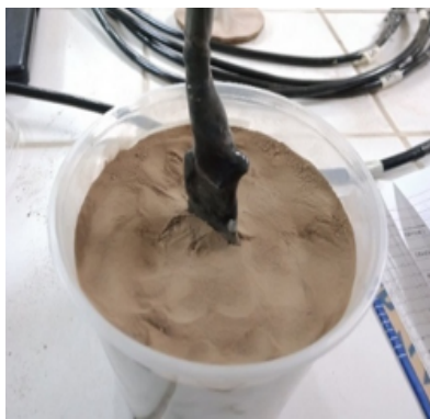
Figure 9. Laboratory calibration of soil moisture sensors.
