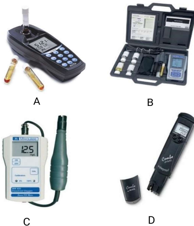
Figure 2. Water quality sampling instruments:(A) V2000 Multi-Analyte Photometer, (B) EUTECH PCD650 waterproof portable water quality meter, (C) MW 600 Smart DO meter, (D) Hanna Combo pH and EC meter
