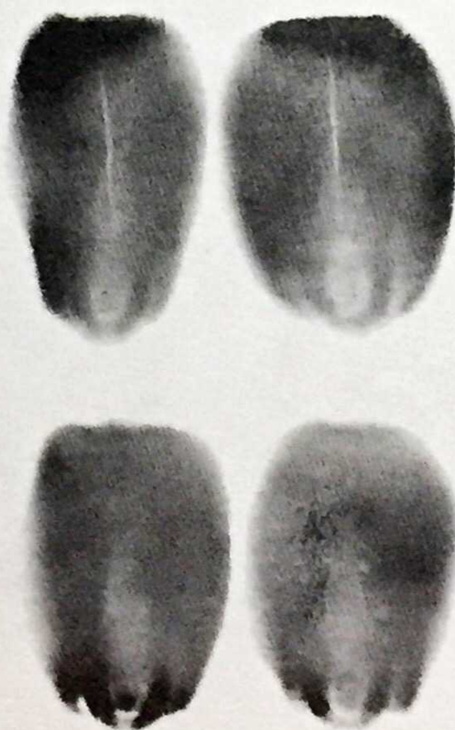
Figure 5. Photograph of maize seeds x-rayed in the longitudinal position. Top: Seeds with cracks seen by both x-ray and visual examination. Bottom: Seeds showing no cracks under x-ray but hairline cracks detected visually.
