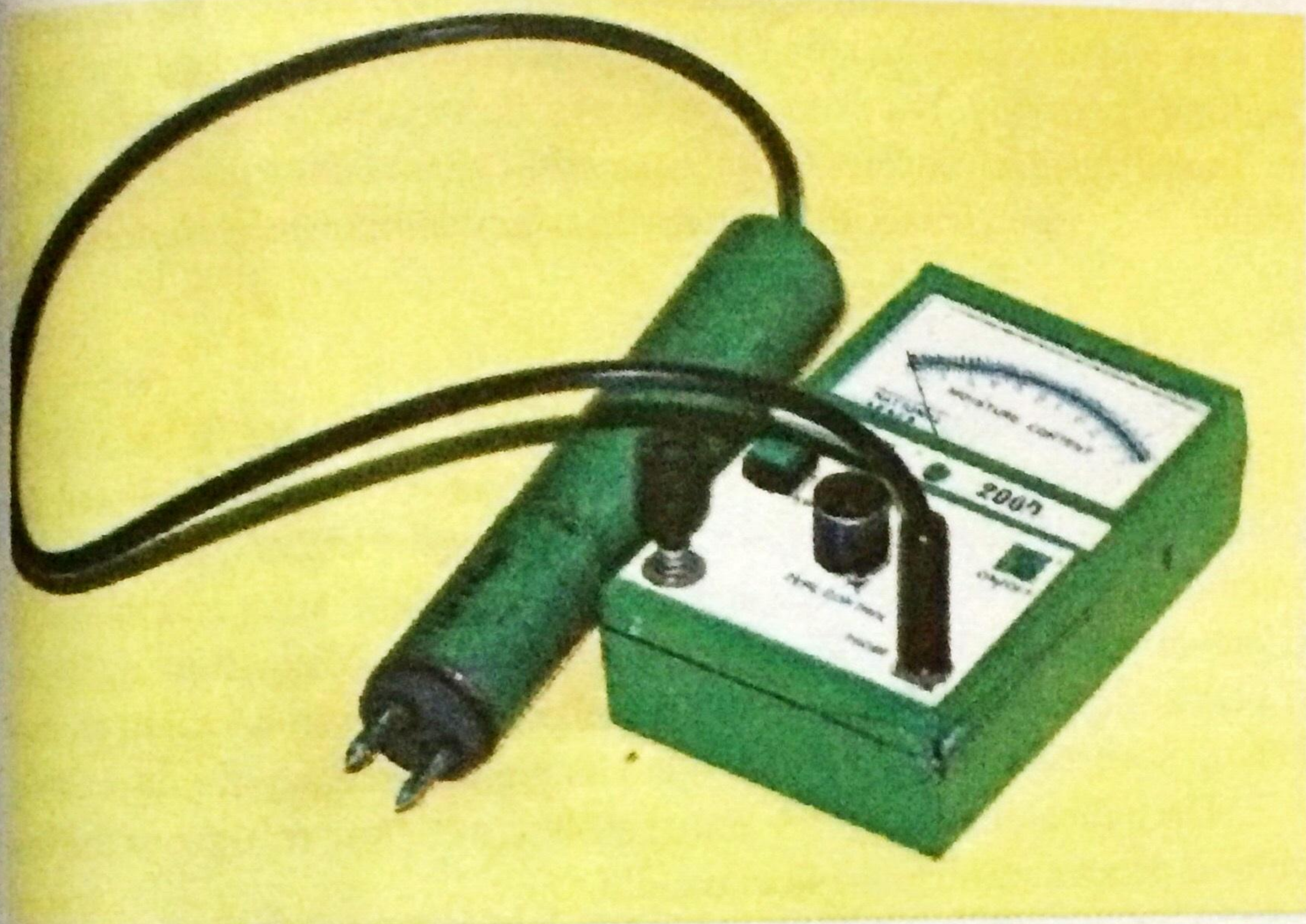
Figure 3. Perspective view of the designed moisture meter for abaca fiber.
