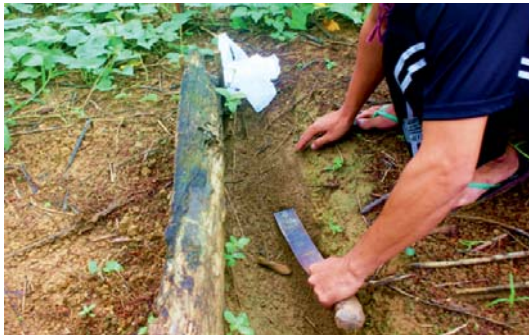
Figure 5. Collection of eroded soil trapped in the trough at the lower portion of each plot for nutrient analysis.
