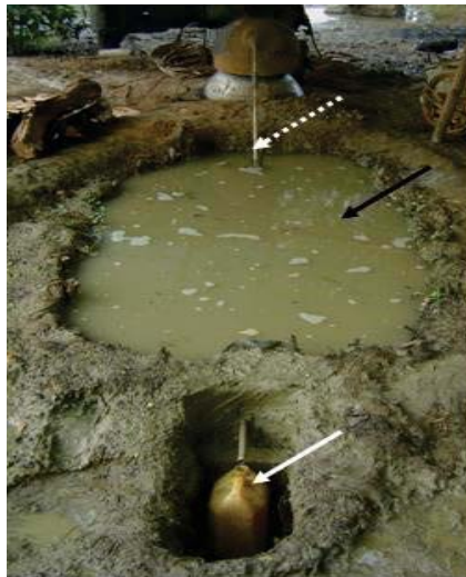
Figure 4. Small scale traditional mahuli distillation process from fermented mahua flower. Dotted white arrow: Metallic pipe connected to the upper vessel, Black arrow: Mud water, through which metallic pipe passes and it helps in condensing vapors to liquid, White arrow: Condensed Mahuli Collecting vessel.
