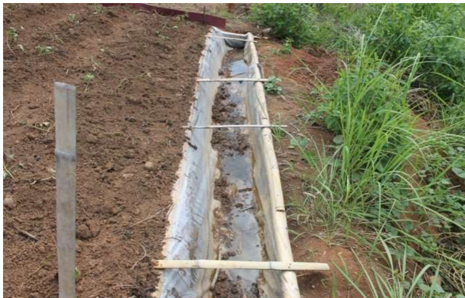
Figure 5. Trench constructed at the lower end of each erosion plot for collecting eroded soil
