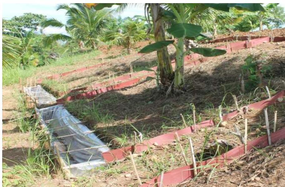
Figure 4. Erosion plots established in the corn fertilization experiment
