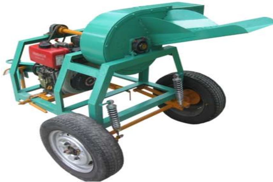
Figure 8. Perspective view of the fabricated plant shredding machine
