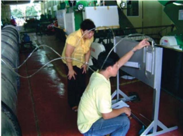
Figure 5. Static pressure measurement using an inclined manometer.
