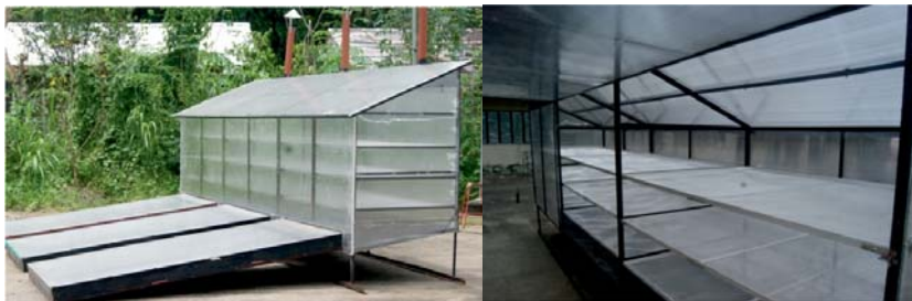
a) Perspective of the solar dryer b) Interior view of the solar dryer
